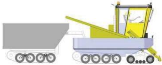
C. Virtual model of an amphibian tracked unit with modified front tracks.
