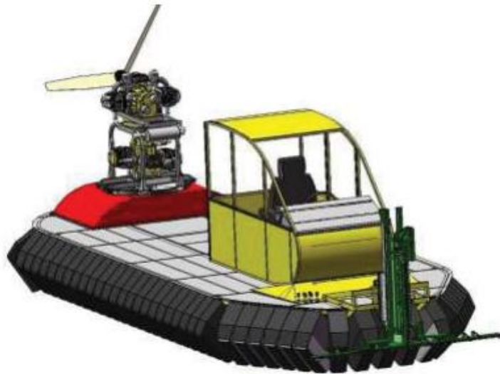
A. Virtual model of the Agricultural Hovercraft Tools Carrier (AHTC) with a T-shape mower.
