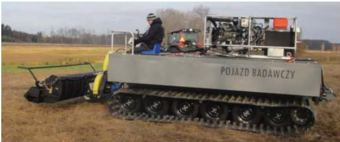
A. The pre-prototype version of the tracked amphibian tractor during field testing.
