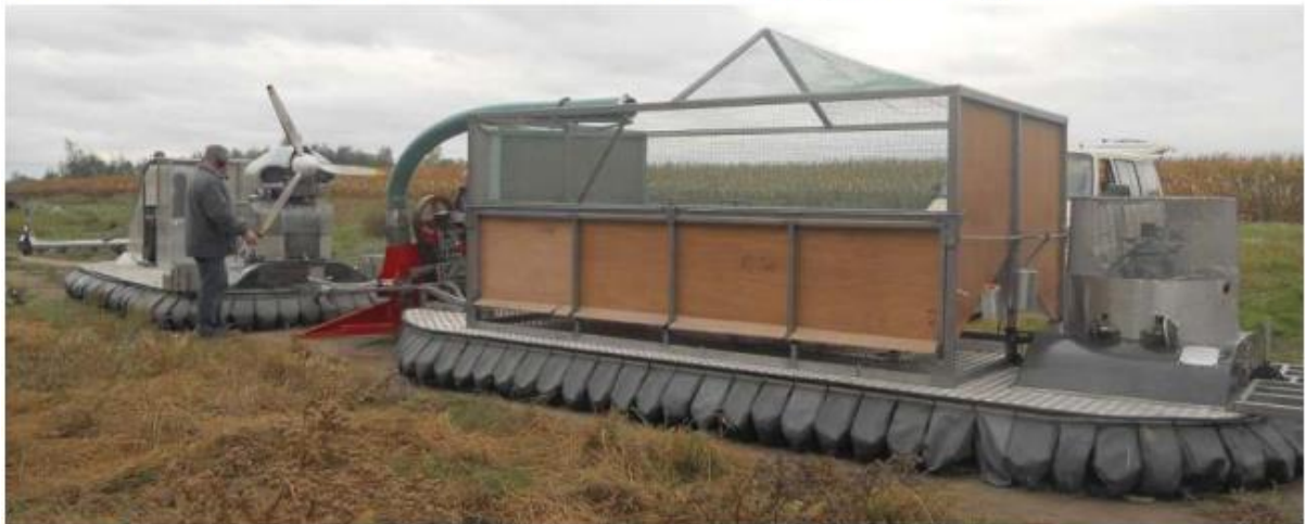
B. The tangible prototypes: the Agricultural Hovercraft Tools Carrier coupled to its Transportation Module.
