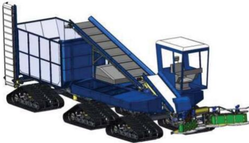
B. Virtual model of an amphibian tracked unit with long tracks, similar to those used on snow groomers.
