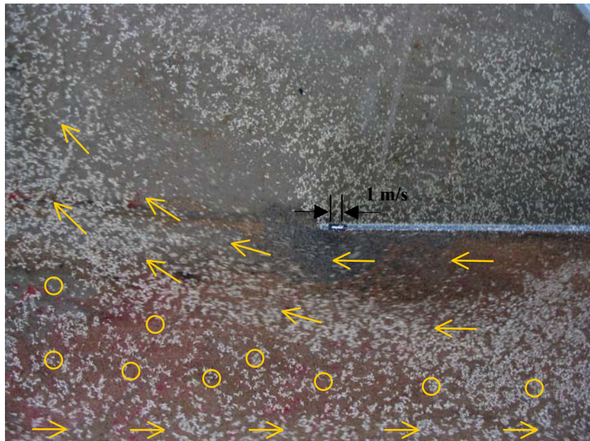
Figure 88 : Entonnement amont (vue A) – Q = 1500 m 3 /s
