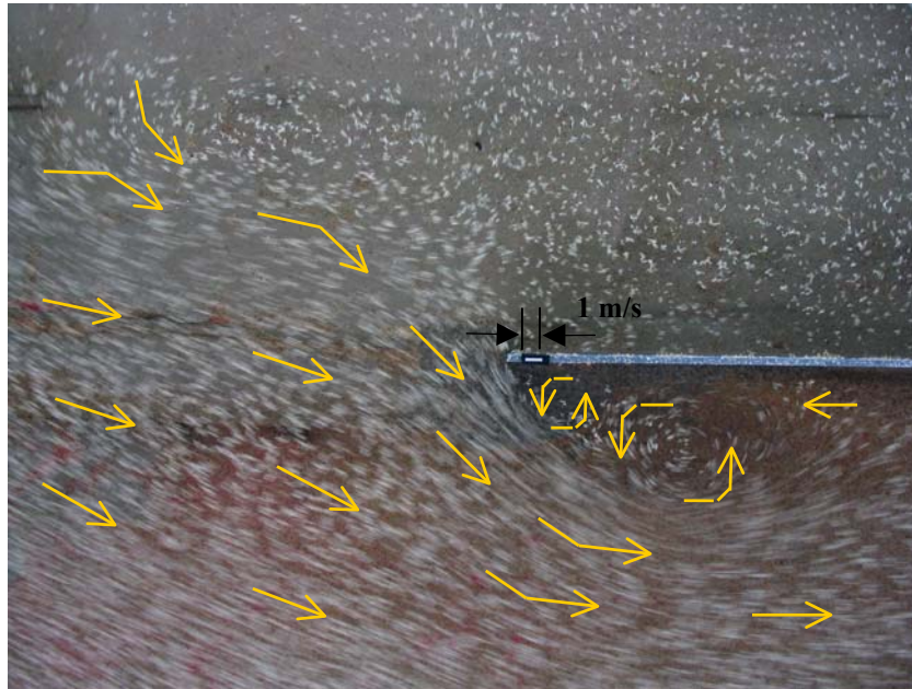
Figure 91 : Entonnement amont (vue A) – Q = 4600 m 3 /s
