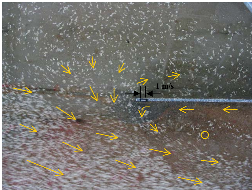
Figure 90 : Entonnement amont (vue A) – Q = 3000 m 3 /s
